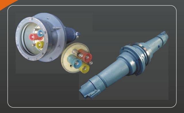
"MEDITRON" make HT PLUG & SOCKET / COUPLERS suitable for use up to 6.6 KV. Each coupler is equipped with silver-plated copper contacts rated up to 400 ampere. MEDITRON's Couplers feature a durable corrosion - resistant aluminium cast / iron shell. The couplers are available for in cable extensions or equipment. The plug & socket is suitable for equipment mounting. The couplers are totally enclosed when coupled, making them flame, dust and weather proof.
