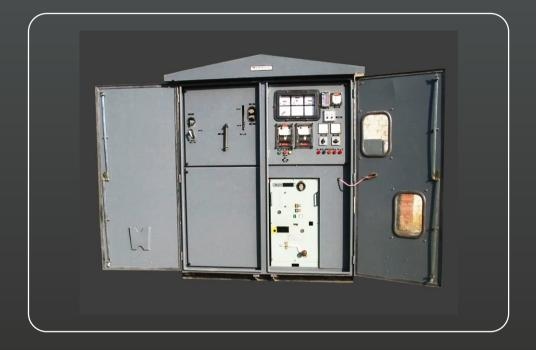
MEDITRON make Field Switch is used in open cast mines for feeding HT power to the mobile mining equipments. The design is robust and suitable for frequent shifting in open cast mines. The enclosure is designed for IP 55 and can be exposed to extreme climatic conditions.
